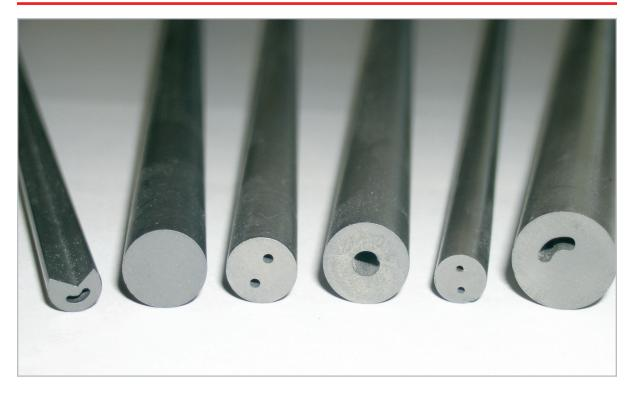
Round, square, rectangular rod, with or without holes, varied shapes with a constant cross section, can be cut to specified lengths, with or without centers. Gundrill blanks can be full-length sticks, cut to length heads, and can have preformed presharpening angles included. Round or other shaped coolant holes including single hole, double hole or kidney holes can be manufactured.
