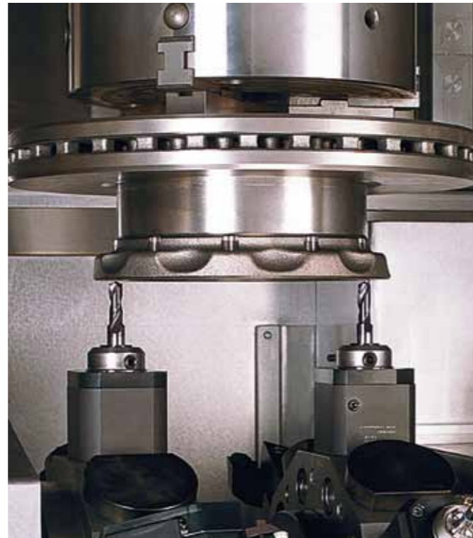
Two drilling turrets and additional Y-axis
