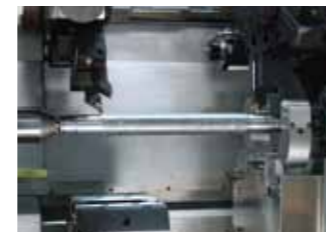
Work area with two upper tool turrets
