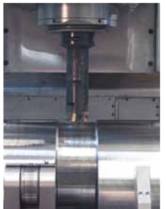
Machining of bearings with B-axis
