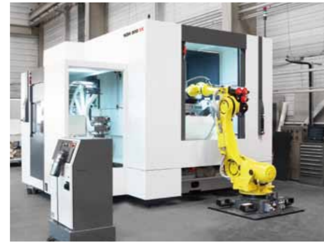
Direct loading of an NBH 800 5X via robot
