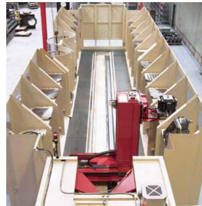
Multi-level pallet storage system with 34 pallets on two levels
