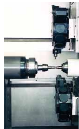
Work area with upper and lower tool turret
