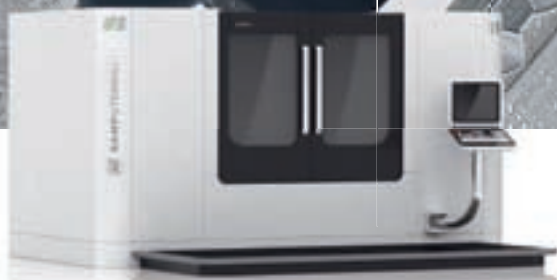
G 500 H for external and internal gears with manually actuated Y axis
