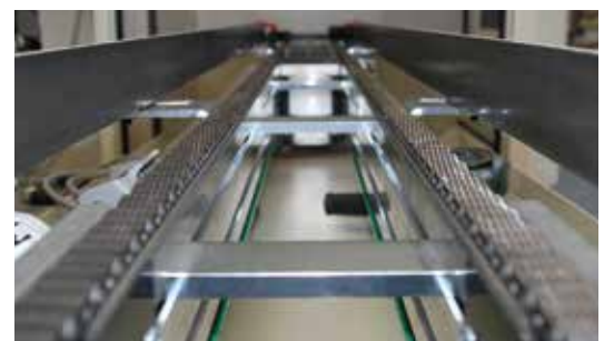
Chain driven conveyor
