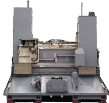
VDM-machine with B-axis and tool carrier
