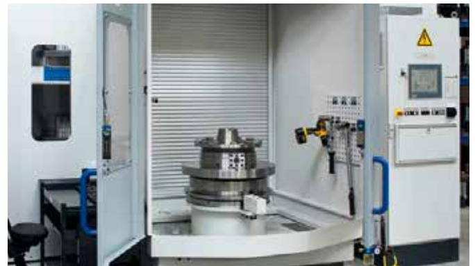
Pallet system with zero-point clamping
