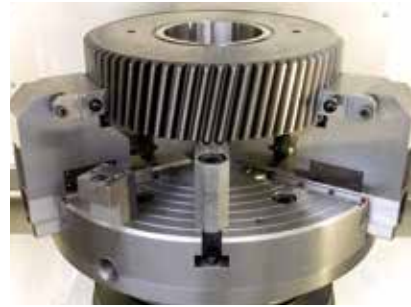
Gear wheel clamped on a VDM 550
