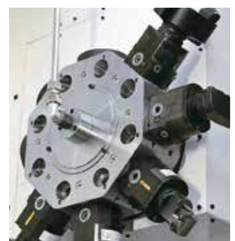
Disk turret with eight tool holders and driven tools
