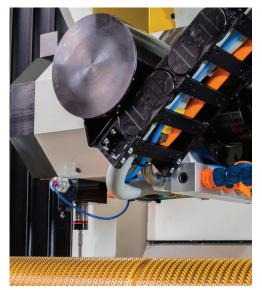
The dual probe system allows for a part probe (shown) to locate the cutting edges of the workpiece and reference it to the machine while the wheel probe locates the grinding wheel relative to the workpiece.
